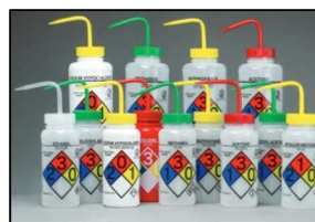
Globally Harmonized System (GHS) wash bottles are vented to prevent solvent drips.
