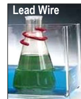
Vinyl-coated lead wire is 300 mm long.
