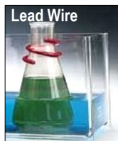
Vinyl-coated lead wire is 300 mm long.
