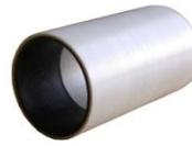
Remove and install prefocused/flanged bulbs safely with this simple tool. Push rubber-lined tube directly onto top of bulb and turn clockwise to install, or counterclockwise to remove.
